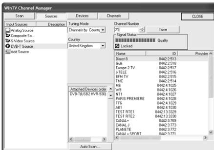
In the WinTV Channel Manager, click on **Sources** then **DVB-T Source**, enter the LCN numbers into the space under **Channel Number** and click on the **Tune** button. The channel number will then be scanned and any channels found will be listed in the channel list below.
